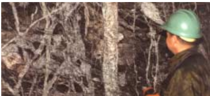
Impressive stockwork system seen in higher grade zones
